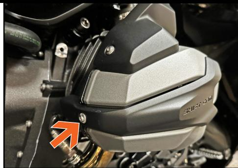
**1** Remove the BMW Spark Plug Cover by unscrewing with a **T30 Torx** Driver. *This Screw will be re-used.* See the **Tab** at the rear of this cover. It engages a **Slot** on the Cylinder Head & the **X-Head** installs in the same way.
