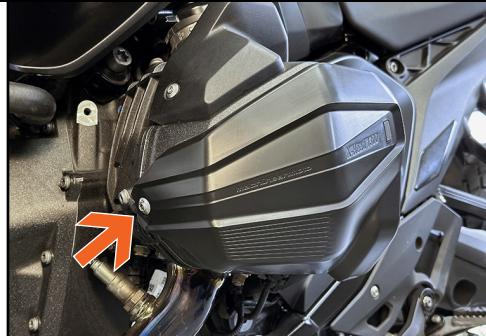
**4** Insert the **T30 Torx** Screw thru the **X-Head** and thread it tightly into the Engine Boss. *A drop of Loctite on the Screw Thread is recommended before re-use.* **Ready to Ride!**
