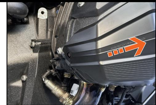
**3** Position the **X-Head** over the cylinder near its forward side, and firmly **slide** it rearward to engage its **Tab** in the **Slot** on the Cylinder Head. Press the **X-Head** toward the rear to **align** its **mounting hole** with the Engine Boss.
